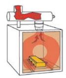
throughout the oven chamber and eliminates cold spots. This precise control of temperature prevents distortion of the part during the process. The primary and secondary water suppression system along with the monitoring of both the oven and afterburner chamber temperatures ensures a safe controlled burn-off.
